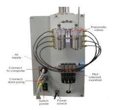
Figure 3 – Typical Pump Connections (back side)
