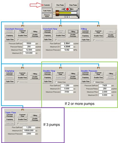
Figure 6 – Software Architecture
