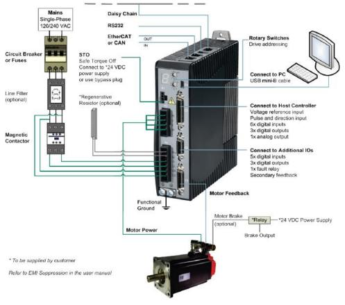
FLEXI PRO-1D5/FLEXI PRO-003 - Servo System Wiring -120/240 VAC, 1-Phase
