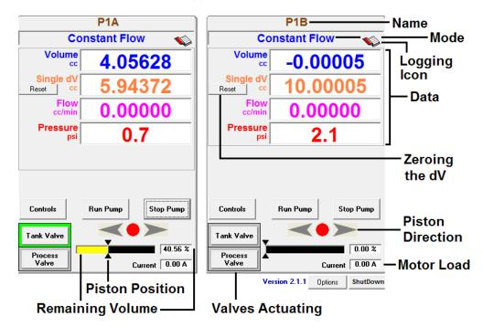
Figure 8 – Standard Main Window for a Two-Cylinder pump
