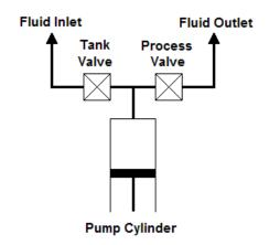
Figure 10 – Standard Pump Cylinder Piping
