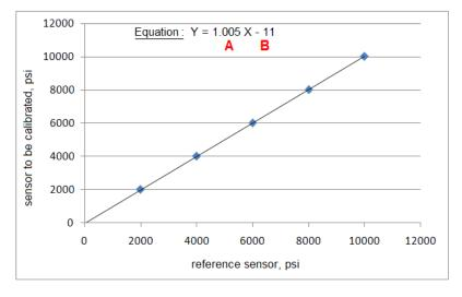
*Figure 28 – Linear Regression for Calibration Procedure* 5.10.2 Pressure Control Calibration
